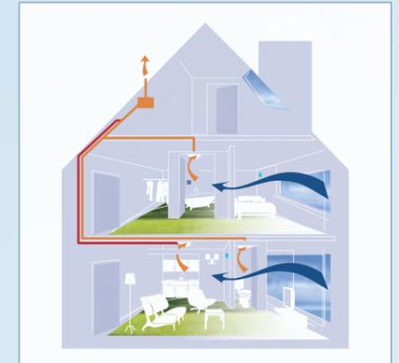
The diagram illustrates a typical "System 3" central extract duct layout, focusing on the 'Best Practice' that the toilet extract is separate to, or positioned in line between the kitchen extract and the extract unit. The unit should only be positioned in the loft, if it is positioned within the heated envelope of the building.
